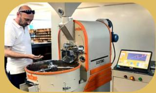
Sizes w x l x h :80\*175\*176 cm Exhaust pipe diameter : Ø168mm Voltage & Frequency : Single Phase 110 / 220V 50hz 60hz Three Phase 380 / 400 50hz 60hz Power : 1.65 kw/h Electric Current (Ampere) 14 Amp Fuel type : Propane, LPG, Natural Gas, Electricity Gas pressure requirement : NG 20Mbar – Propane, LPG 30mbar Source Gas Pressure : 1-4bar
